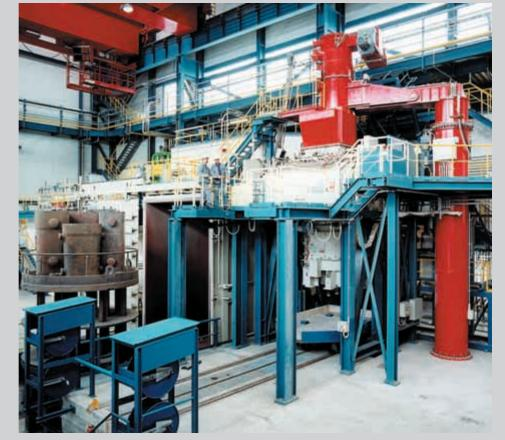
ThyssenKrupp VDM GmbH operates the world's largest VIM furnace, type VIDP, at its Unna melting plant.
