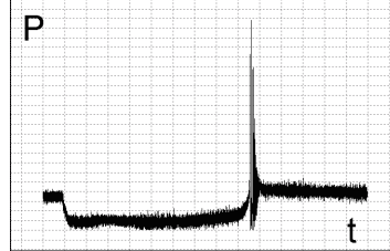
Ordinary diaphragm valve shut-off diagram – EXCESSIVE WATERHAMMER
