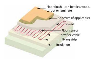
Here the insulation is laid on top of the concrete slab, followed by the heating cable. The cable is covered with a minimum of 65mm\* sand and cement screed. The chosen floor covering is then laid; this can be tiles, wood, laminate, carpet or vinyl.
