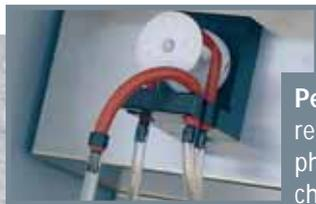
**Peristaltic pump** for the reagents dosing in the photometric cell, equipped with check for the alarm transmission
