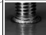
Brand-new and patented stud welding up to M16 in radially symmetrical magnetic fields (Patent No. 10 2004 051 389)
