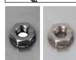
Nut welding of standard M8 - M12 nuts in radially symmetrical magnetic fields on punched and non-punched sheet metal
