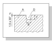
The hotflex<sup>®</sup> can be put directly into a slot of a manifold or knocked in with a plastic hammer.
