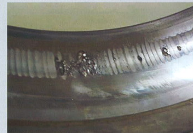
Damage to ball bearing raceway
