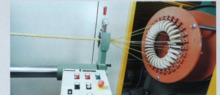
State-of-the-art stranding machinery at the Windsbach factory
