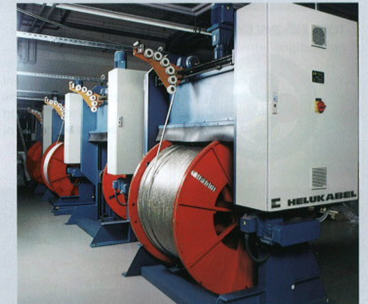
Reeling after braiding at the Windsbach factory
