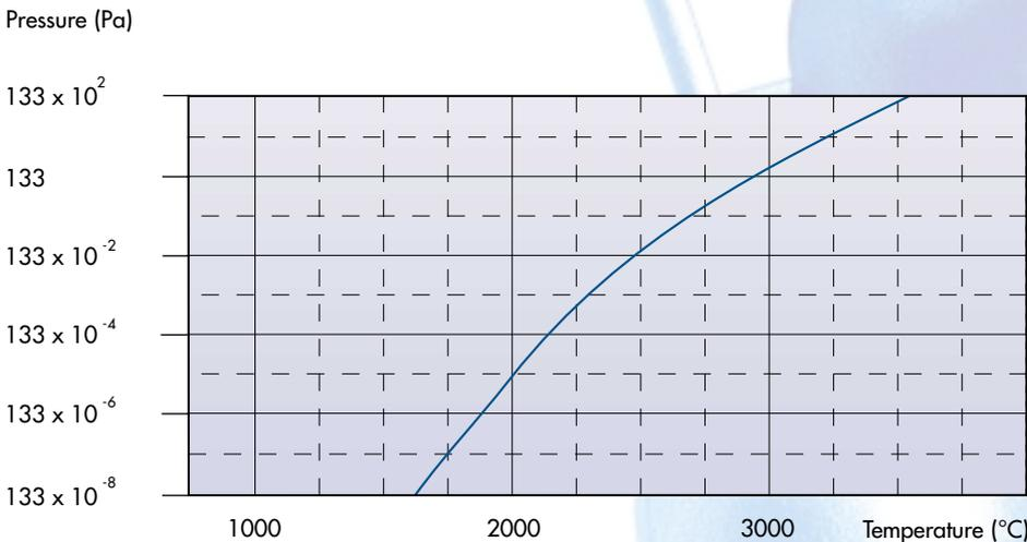
Carbon vapor pressure during high-temperature operation
