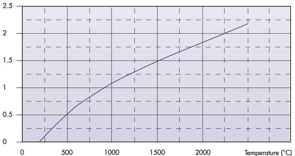
The increase should be added to the typical value of the linear expansion coefficient at 20-200 °C.
