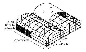
All Conley's greenhouses feature rollformed steel. Each truss assembly is made from one rollformed component, no splices required, between peak to gutter connection.
