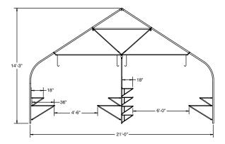
The Retail Mart is designed to easily erect multiple, gutter connected units to make it ideal for future expansion. All Retail-Mart Greenhouses are engineered to meet 70 mph wind and 10 pound live load per the UBC Building Code. For an additional expense, your structure can be designed to meet any building code requirements for live and/or wind load. Call IGC customer service for pricing on any custom requirements.
