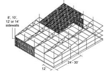
All Conley's greenhouses feature rollformed steel. Each truss assembly is made from one rollformed component, no splices required, between peak to gutter connection.
