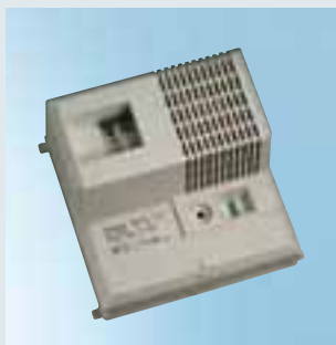
Fuse box with integrated converter H With B 10 A circuit breaker and build-in 12 V mains adaptor performing at 2 x 9 A DC current
