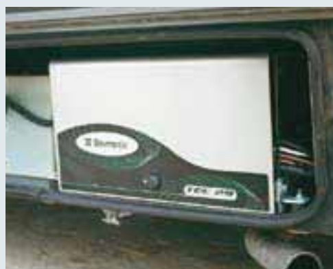
The TEC 29 is mounted underneath the vehicle's chassis or tucked away in a ventilated storage box. The installation of the exhaust is flexible.
