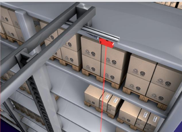
Reliable detection of **stretch-wrapped** pallets.
