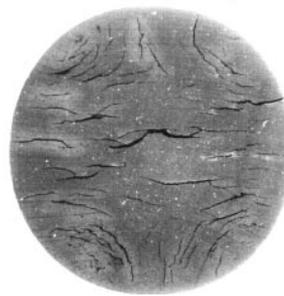
This phenomena is known as Explosive Decompression (ED). Cracks and blisters may be evident on the surface of the seal, they may be internal, or they may only be detected by magnification.
