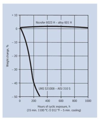
Fig. 2 - Scaling resistance of Nicrofer 6023 H compared to AISI 310 S.
