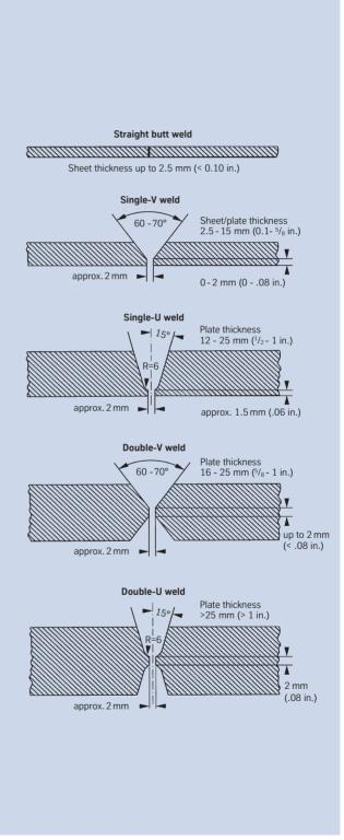
Fig. 3 – Edge preparation for welding of nickel alloys and special stainless steels.
