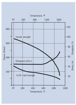
Fig. 1 – Typical short-time properties of solution annealed Nicrofer 6023 H at elevated temperatures.
