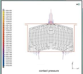
contact pressure distribution after installation ( p = 0 bar)
