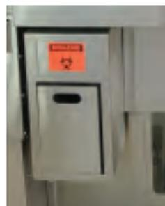
**Ventilated Trash Container:** 13.5"x 8-3/4" x 13" Deep, removable, 5 gallon capacity. Self supporting, the trash container is provided with a spring activated trash chute and automatically connects to the ventilation system and can be moved within minutes from the right or left inner skirt area. Connects to grossing station ventilation system
