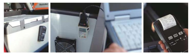
For the sake of continuous, tamper-proof temperature recording the data logger is firmly integrated in the cooler. Data can be transferred to a laptop computer via a data cable with infrared interface – or printed out directly using the attachable printer.
