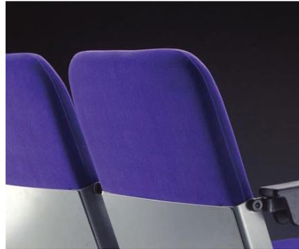
Cast aluminium sides finished in powder epoxy paint support the seat, back and armrest assembly. The seat and back pivot on polyamide bushings that require no maintenance. The folding mechanism relies on gravity involves no springs. This ensures maintenance free, extended durability. At the bottom, the sides fit onto, and are fastened onto, the tubular foot structure.
