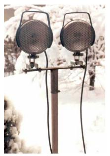
The devices EL65... and EL66... can be equipped with alternators for 110 W power output to power the floodlights. The two halogen lights with 55 W respectively are mounted on the 2 m mast. They can be swivelled and the connecting cable has the suitable connector for the socket of the alternator. The mast slides into a standpipe mounted to the device.
