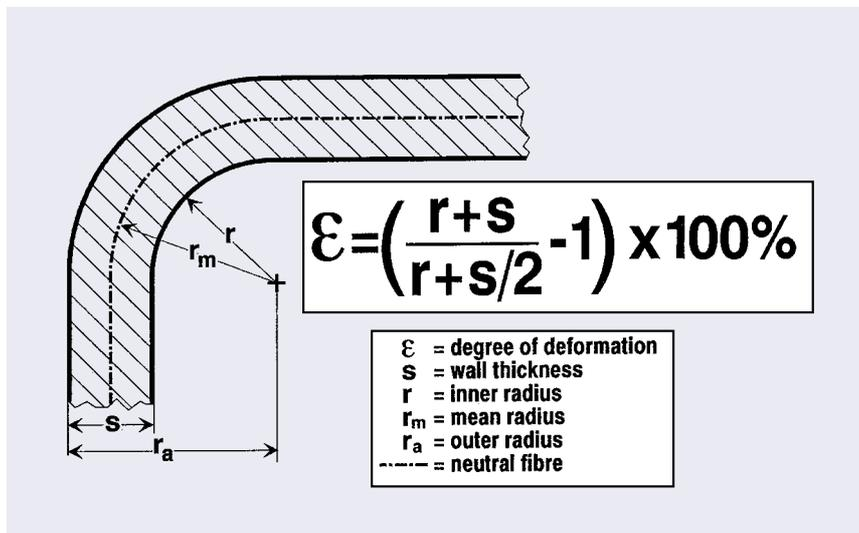
Fig. 1 – Calculation of the degree of cold deformation in bending
