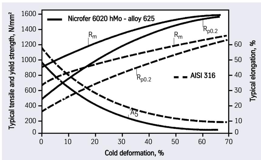
Fig. 2 – Effect of cold deformation on mechanical properties
