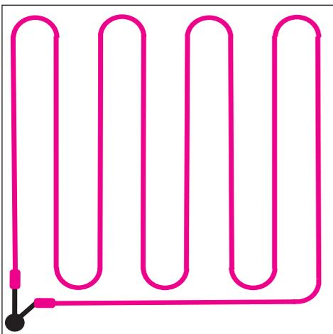
9. The heating cable or mat may not be cut/shortened or exposed to strain in the areas of the cold cable.
