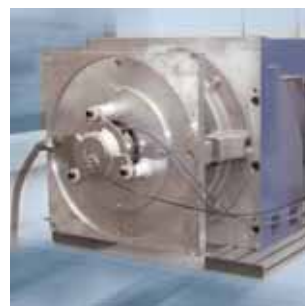
Test rig for grounding contacts. Measurement of the heat development of the carbon brushes
