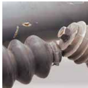
Broken pantograph drive spindle, caused by heavy external interference
