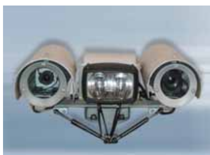
Using the camera mounted on the measuring train, the performance of the pantograph is observed during operation. Defect spots are recognized early
