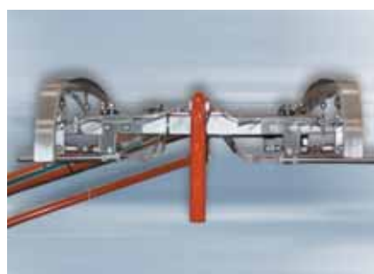
Detailed view of a test pantograph. Easily visible on the left and right under the collector strips: pitot tube for measuring wind speed
