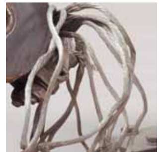
Torn current connectors on pantograph
