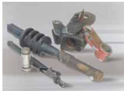
Dependent upon length of use and operational demands: worn out bearings connections and current conducting parts
