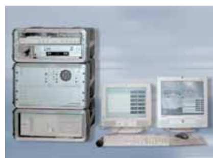
Live transmission during operation. Live pictures appear on the screen in the measuring train: position and behavior of the overhead wire, contact pressure etc.
