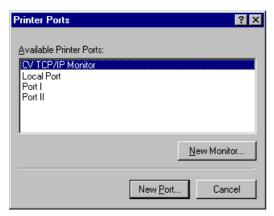
Select **CV TCP/IP Monitor** from the list of **Available Printer Ports**, activate the **New Port** button and the Wizard for adding a Standard TCP/IP Printer Ports appears.
