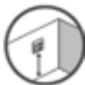
When Devireg™ 535 is used as a room sensor, installation height should typically be between 80-150 cm.
