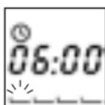
By pressing the ● the start time of the period starts flashing. You change it with the arrow buttons ▲▼ in increments of 15 minutes.
