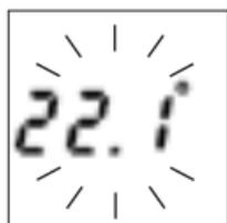
Use the arrow buttons ▲▼ to either increase or decrease the temperature. The temperature is changed in increments of 0.1°C.
