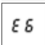
Error code 6 - Floor sensor disconnected
