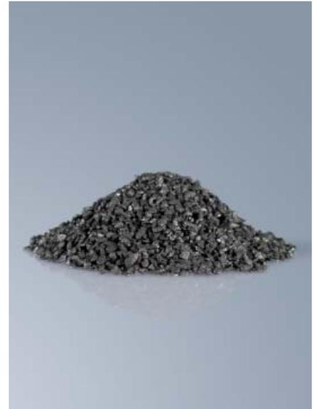
Zirconium diboride –  $ZrB_2$  1-3 mm
