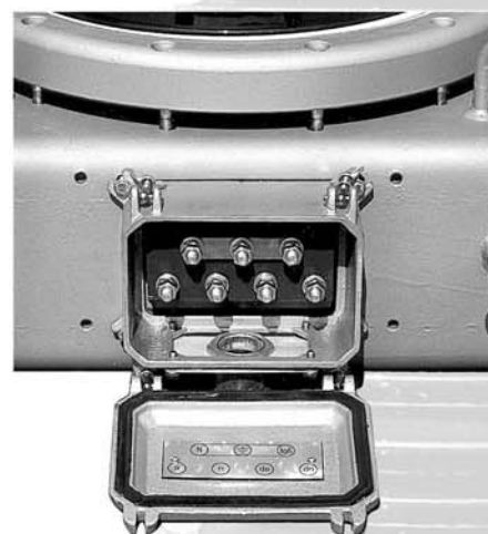
Secondary terminal box
