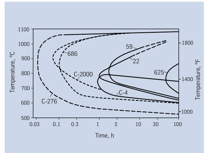
Fig. 2 – Time-temperature-sensitization (TTS) diagrams of nickel-chromium-molybdenum alloys tested according to ASTM G-28 A. Areas to the right of the curves indicate intergranular corrosion  $>50\mu\text{m}$  (.002 in.)
