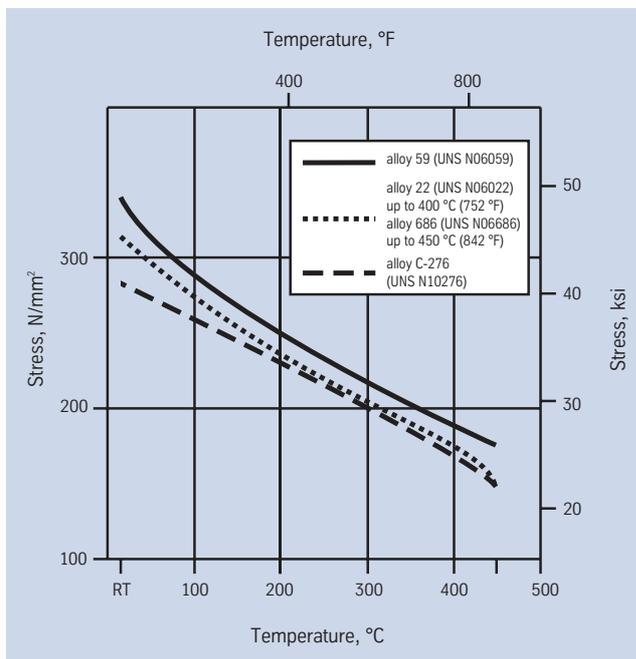
Fig. 1 –  $R_{p0.2}$  yield strength of Nicrofer 5923 hMo in comparison with other nickel alloys.
