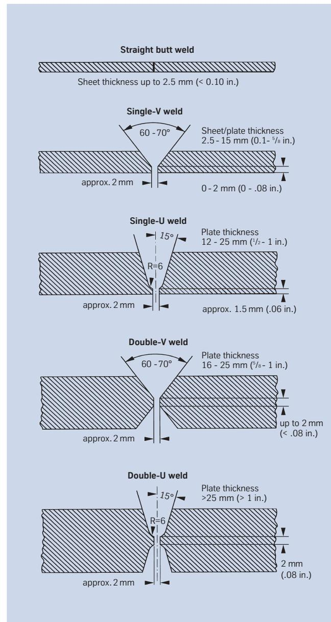
Fig. 5 – Edge preparation for welding of nickel alloys and special stainless steels.
