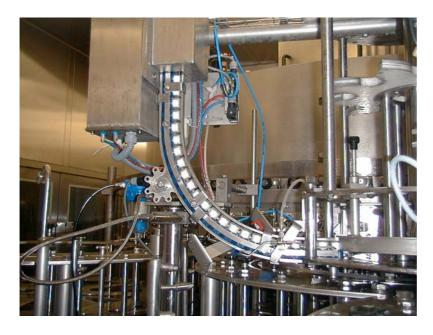
UVATEC used for the disinfection of screw caps in the beverage industry
