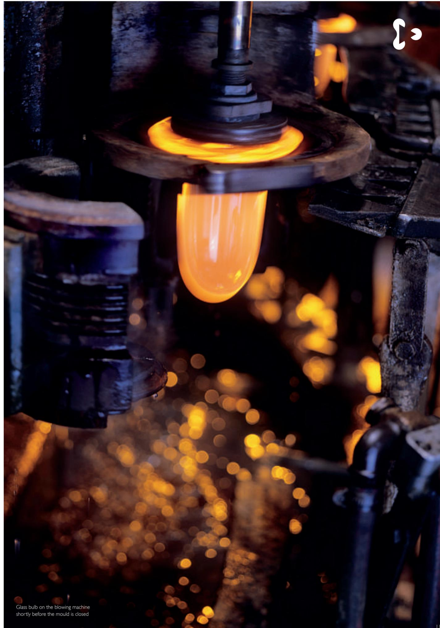
Glass bulb on the blowing machine shortly before the mould is closed
