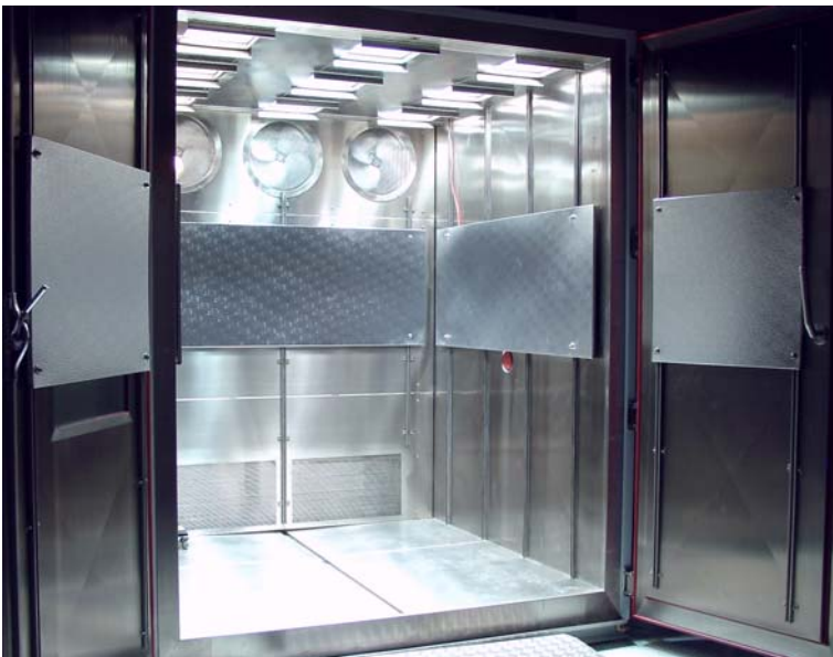
Climatic chamber with 9 SOL 2000 units
