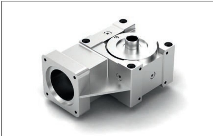
The demand for an absolutely force-locking and virtually torsion free connection between the gear unit and the output shaft, especially in intermittent operation, is met by a new gear version designed for shrink disk fastening of the output shaft.
