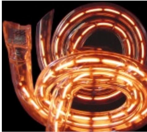
**When riveting two components together, an Omega emitter only has to heat the rivet and not the whole component**
