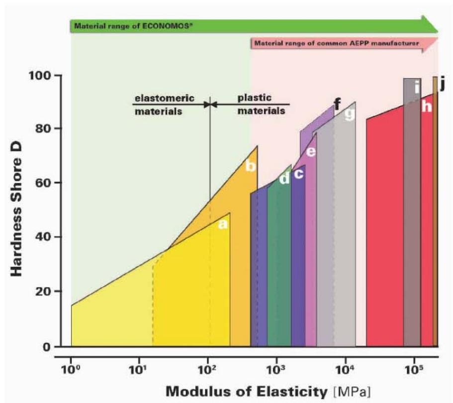
Fig.: Range of hardness as a function of modulus of elasticity for various AEPP material groups
