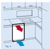
the shutter at the top rear of the refrigerator. Of course, you can also install your refrigerator at eye level. In that case, there should be enough space for air intake between the floor and the wall. Air outlet is via the shutter at the refrigerator front **(Fig. 3)**.
