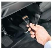
Connection to the accelerator via T-plug
