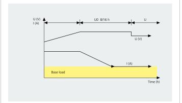
To prevent overcharging when power is drawn from the battery while charging, the duration of the UO phase is limited.
