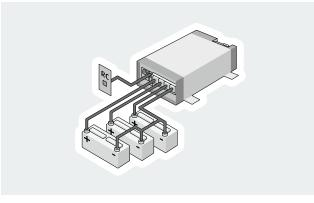
When two or more batteries are used independently of one another, the load on them will be different and so will the required extent of recharging.
