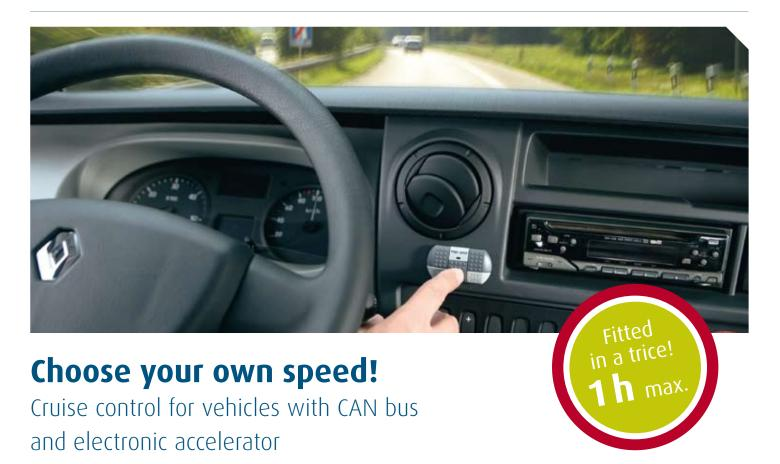
In more and more vehicles, the entire engine management is done by highly complex electronics. The individual control units are networked by CAN bus links, and the pressure on the accelerator pedal is transmitted electronically. Conventional cruise controls with servo unit cannot usually be used in such models.
