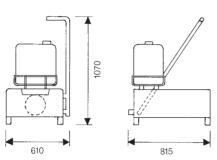
Technical DataDimensions:815 x 610 x 1070 mmWater feed:R 3/4"Drain:R 11/2"Electric mains.400 V, 50 HzPower:0,25 KWProtection:IP 65
