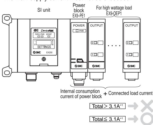
**Supply current between SI unit and power block**
