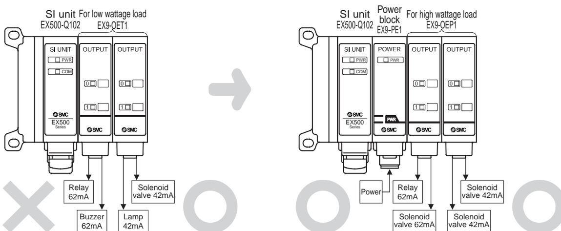
(5) The number of output point when the power block is used
