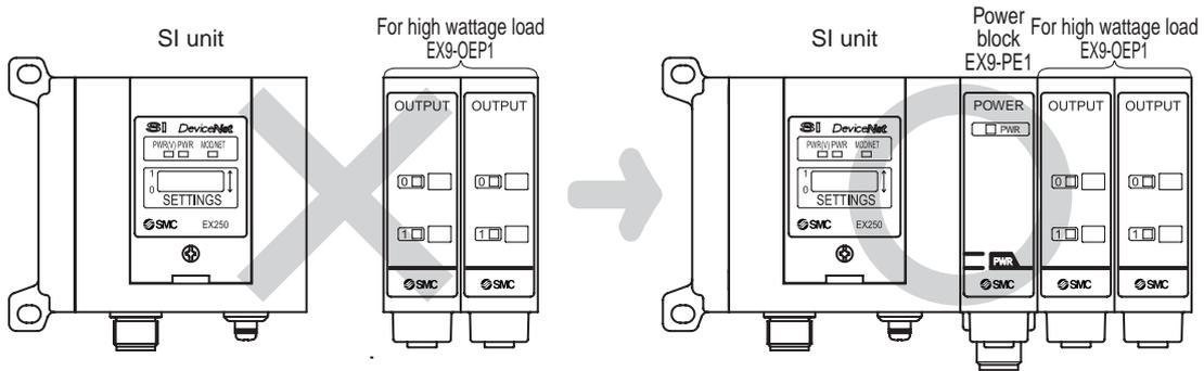
(2) Position of output block for high wattage load
