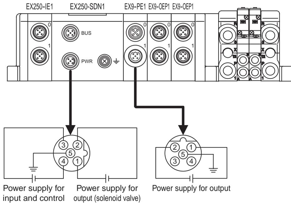
B. The supply of power from power block connector to SI unit.
