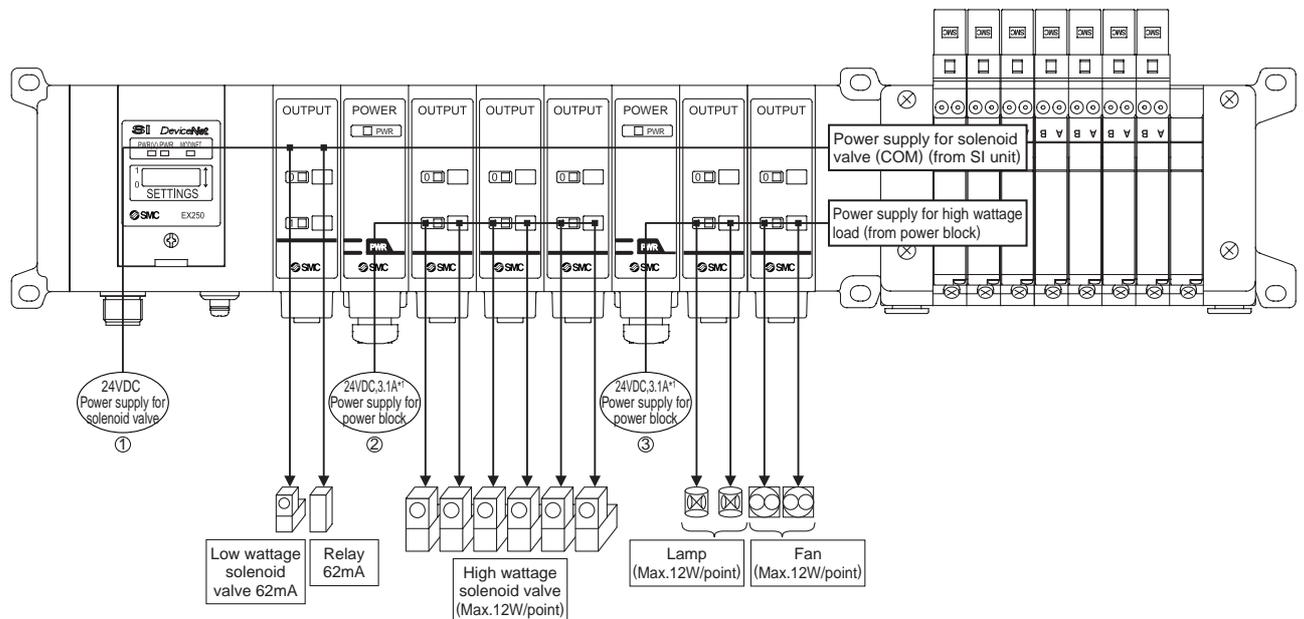
Fig. Power supply system diagram for output block
