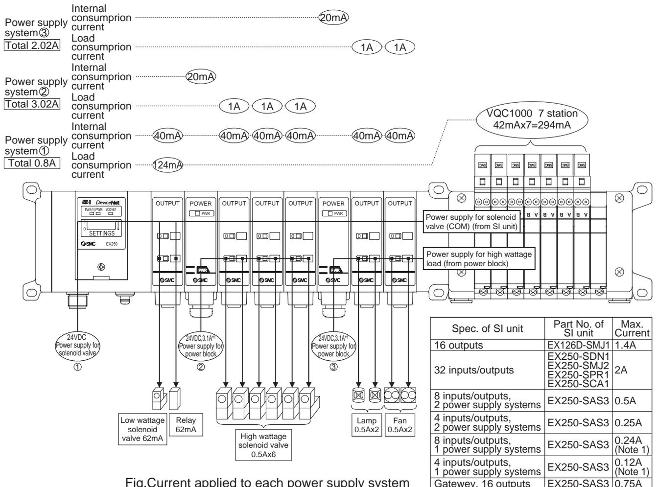
Fig. Current applied to each power supply system
