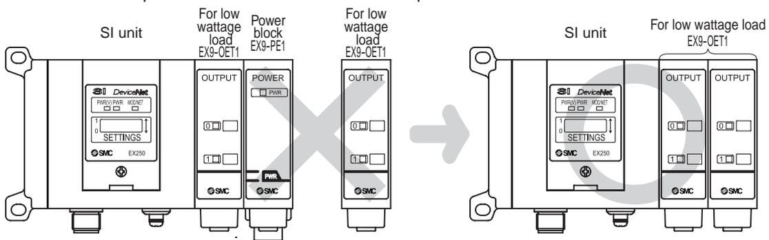
(4) Load connected to output block for low wattage load
