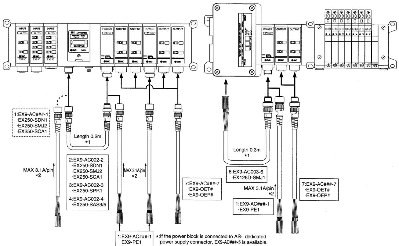
\*1: This cable is a bypass cable used for the layout where the power block is located to the right of the SI unit.
