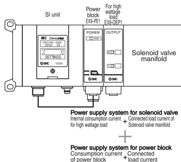
\*1: If max. supply current (3.0 to 3.1A) is applied for operation, do not make the ambient temperature exceed 40°C and bundle the cable.
