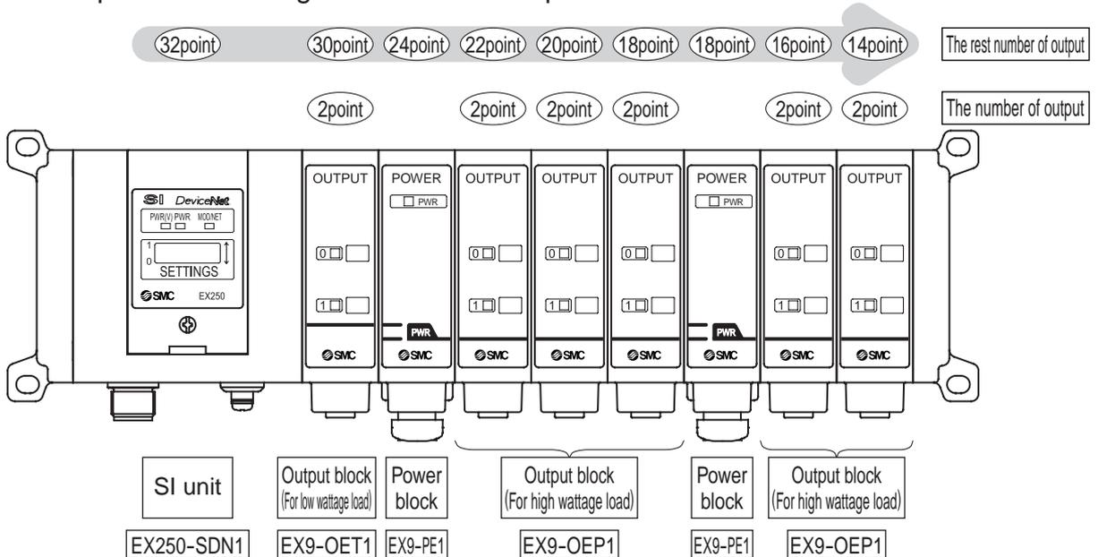
Fig. Example of calculating the number of output
