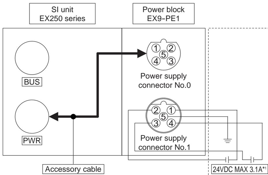
\*1: If max. supply current (3.0 to 3.1A) is applied for operation, do not make the ambient temperature exceed 40°C and bundle the cable.
