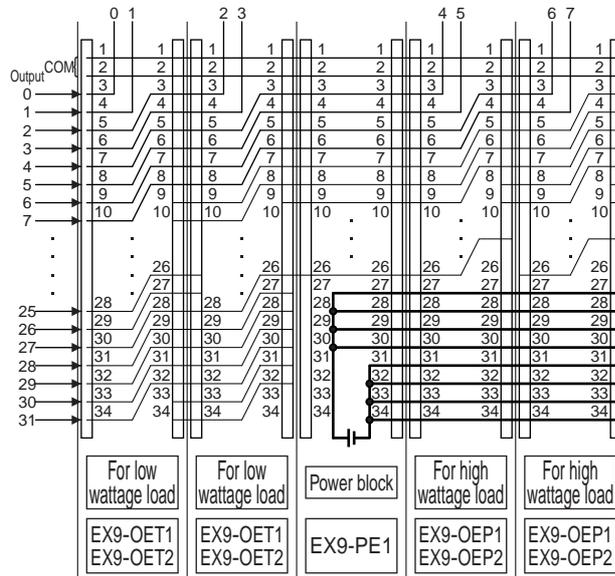
Fig. Connector wiring between output blocks
