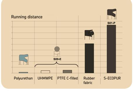
Test results of the reciprocating clear water test rig
