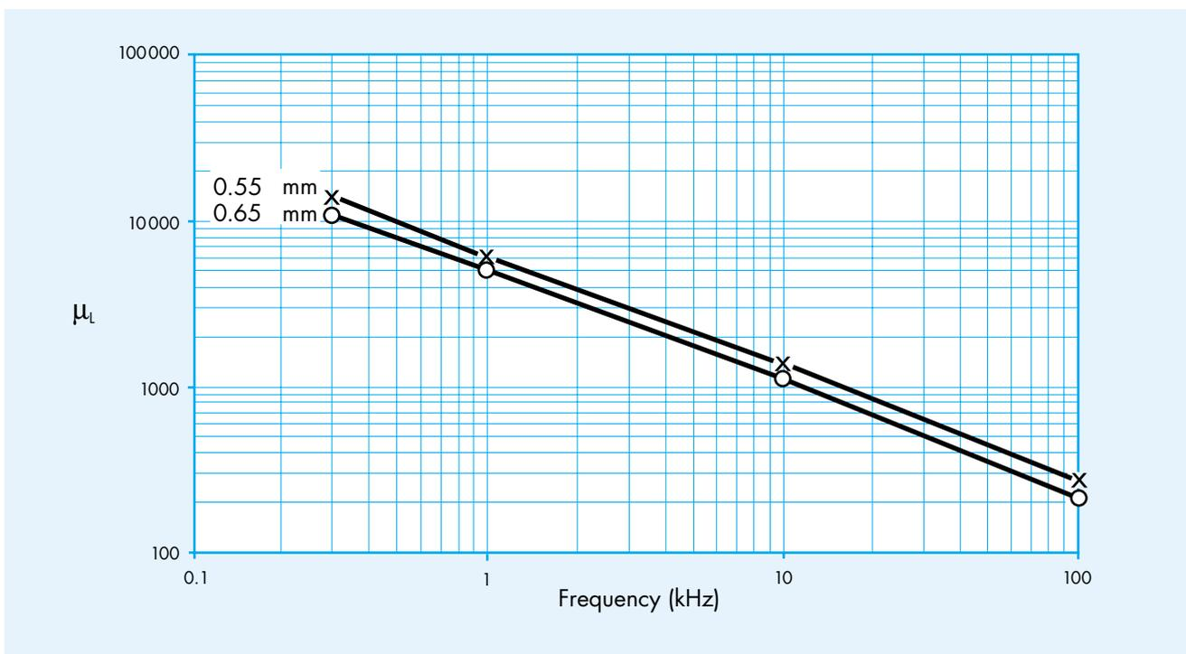
Figure 6 - Typical curves of the inductance permeability  $\mu_l$  of Magnifer 8105 So in relation to frequency and thickness.
