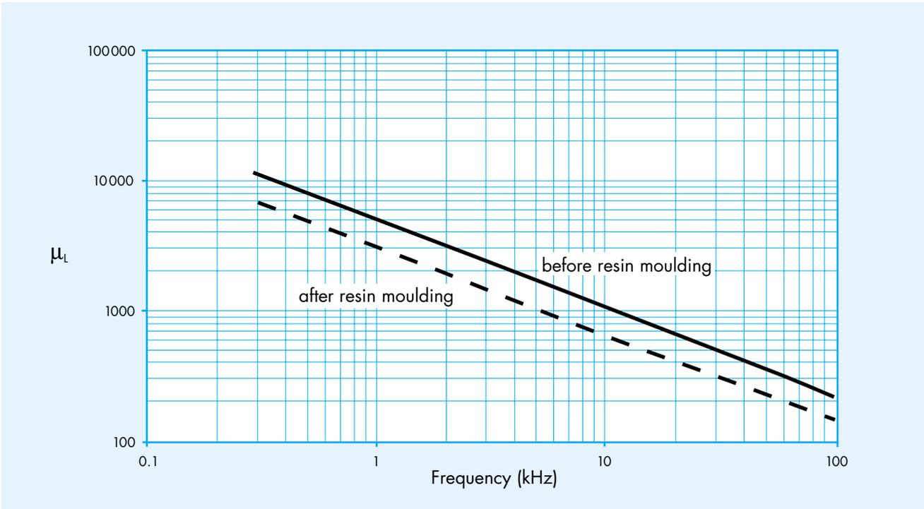
Figure 8 - Typical curves of the inductance permeability  $\mu_L$  of Magnifer 8105 in relation to frequency before and after resin moulding measured using stamped rings of thickness 0.55 mm annealed for 3h at 1050 °C.
