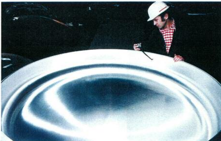
Roll-clad boiler end
