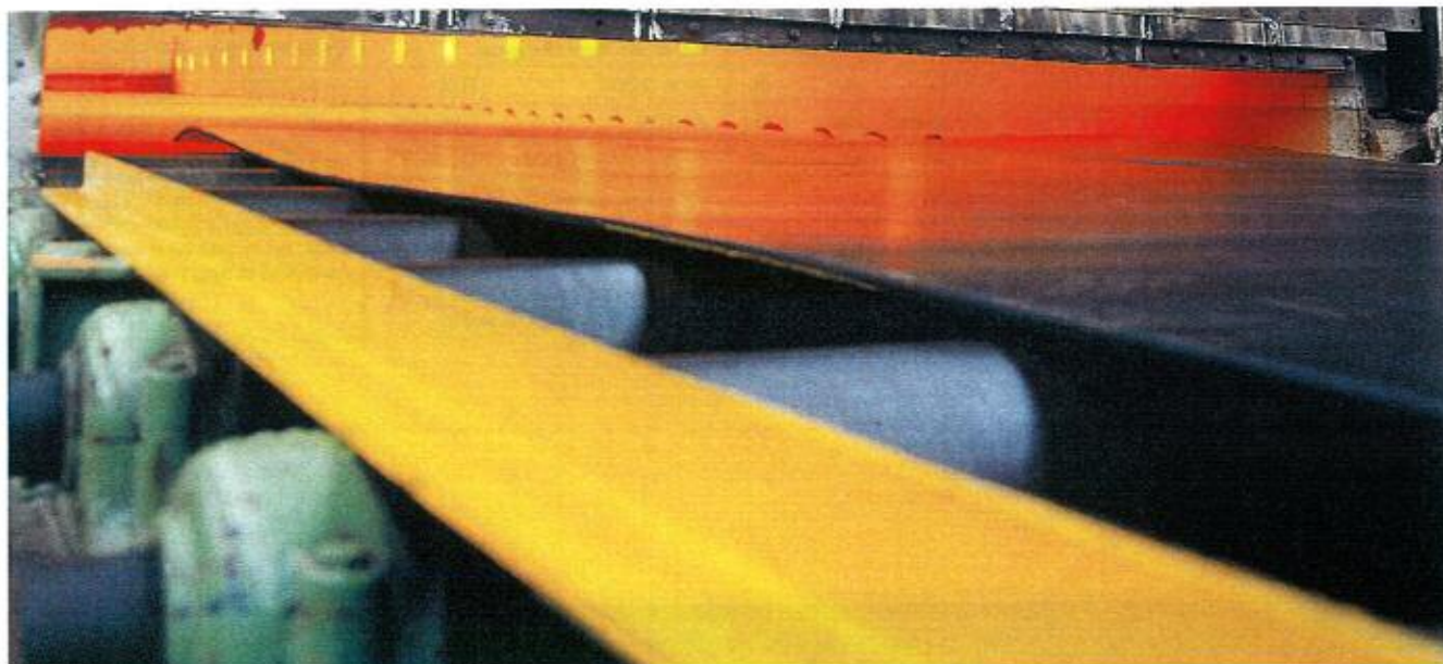
Gas-fired continuous roller hearth furnace with integrated programmable air/water cooling line.
