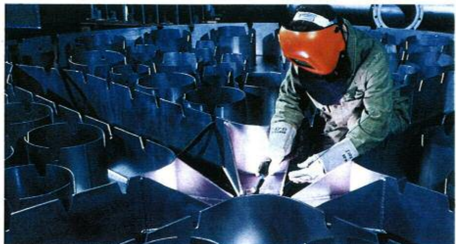
Distributor system of a sulfuric acid plant in Nicrofer 3033-alloy 33. Operator: Norddeutsche Affinerie, Hamburg. Process equipment manufacturer: Franken GmbH, Oberhausen
