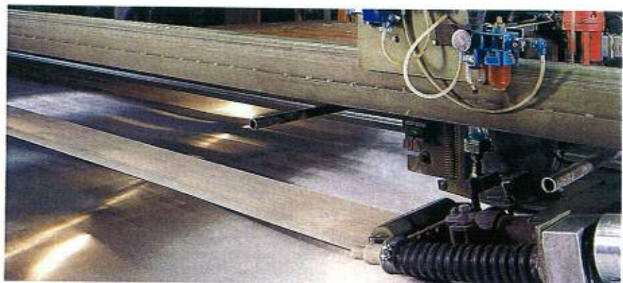
Computer-controlled continuous belt-type surface grinding machine for large sheets in sizes up to 3000 x 8200 mm (10 x 27 ft).
