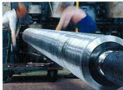
At furnace temperatures up to 1 200 °C (2 200 °F), the previously used water-cooled asbestos rollers were replaced with non-cooled longitudinally welded rollers in Nicrofer 6025 HT – alloy 602 CA.
