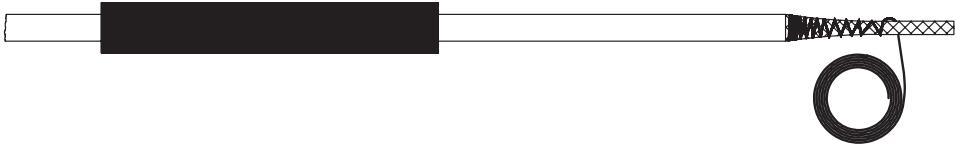
13. Pull the large crimp tube B over the copper protection screen and squeeze the end tight. Apply heat starting at the end so that the air is forced out of the crimp tube. Make sure that the glue is running out from the end of the crimp tube before stopping.
