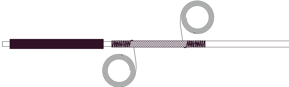
7. Pull the large crimp tube A over the copper protection screen making sure that the tube overlaps equally at both ends.
