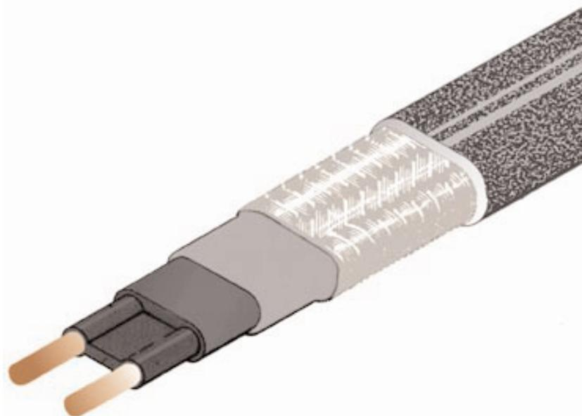
The Devi Pipeguard is a self-limiting parallel heating cable. The power output of the conductive core material increases or decreases in response to ambient temperature changes.
