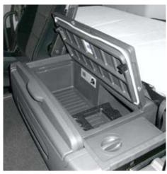
Shown as built-in solution: Dometic cooler for Actros MP2/MP3
