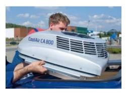
Use existing mounting holes when fitting the new roof air conditioner
