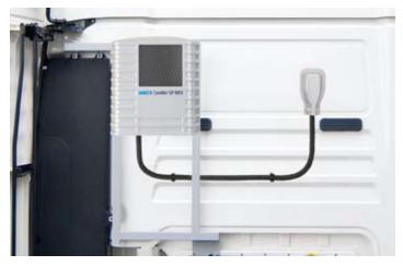
Quickly done: installation and connection of the condenser unit. The condenser fastening frame uses the vehicle's existing fastening points.
