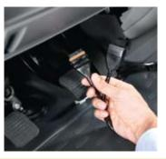
Connection to the accelerator via T-plug
