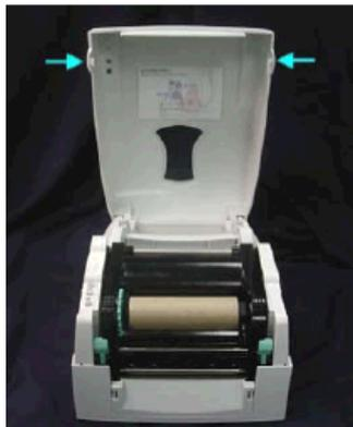
Loosen and then lift the upper print mechanism by pressing the locking tenons.
