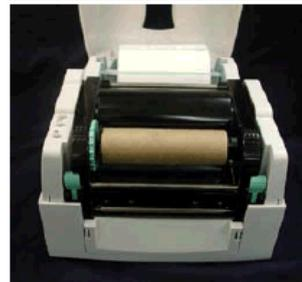
Loosen and lift the upper print mechanism by pressing the locking tenons.
