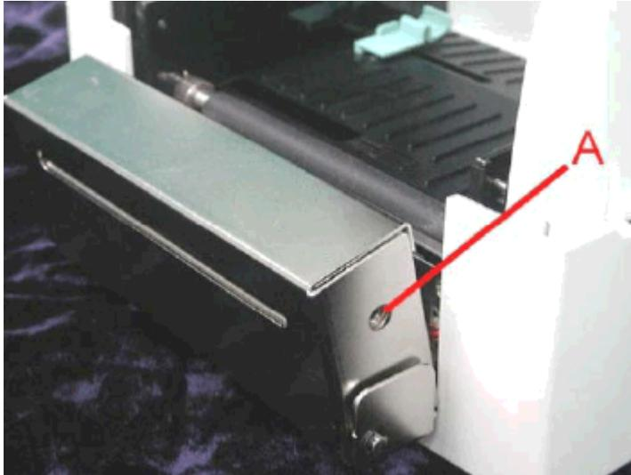
A cutter adjusting hole is present on both sides (where A is pointing to).
