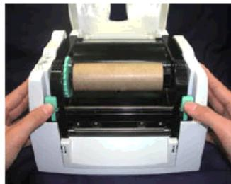
Feed the label through the two label guides to the tear-off bar.
