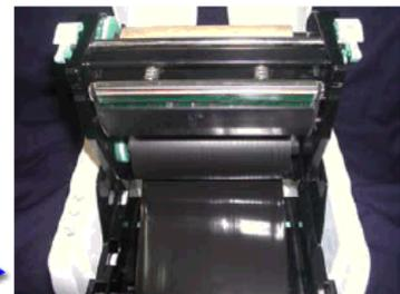
Feed the ribbon from the ribbon supply shaft under the printhead.
