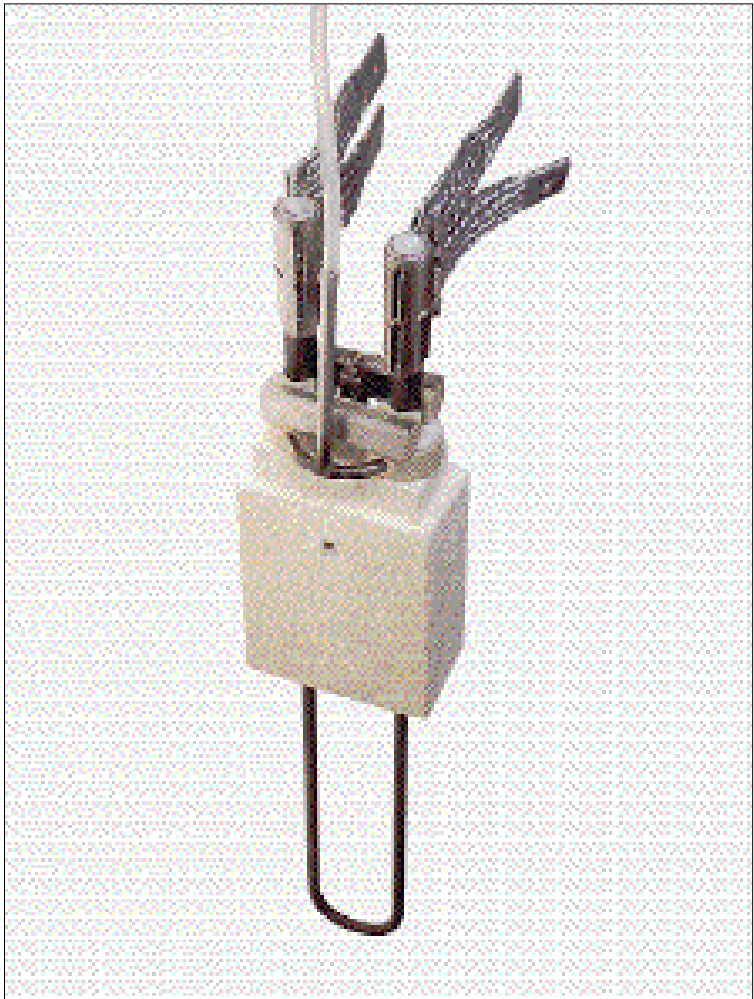
Fig. 43 Element holder and anchor system — Air cooled design.
