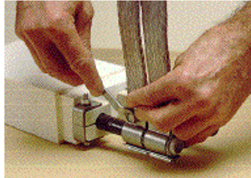
6. When determining the position of the element holder, it is of the utmost importance to ensure that the tapered transition between terminal and heating zone comes fully below the hot face of the furnace lining (10) (g Fig. 47, page 70). If not, there is a risk that the part of the heating zone which is inside the lining may become overheated.
