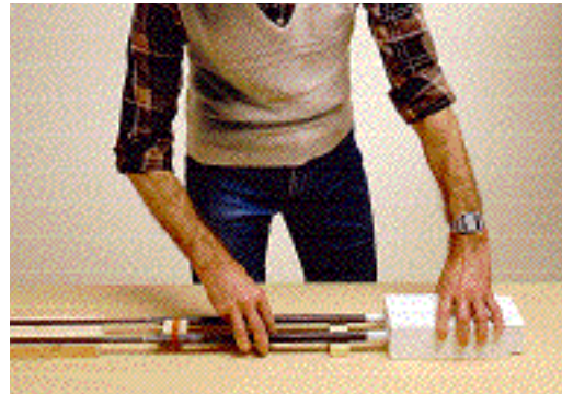
3. The element is placed horizontally on a table and the terminals are carefully inserted in the holes in the passage brick ensuring that the correct length of terminals are protruding from the top of the brick.
