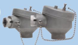
This housing is available in SS 316, and is economically priced to meet to DIN B dimensions and requirements. It can accommodate a medium sized temperature transmitter or terminal block, 50 mm in diameter. The PGI6 version only comes with a cable gland. The processide dimensions are identical to the DIN B head, so they can replace them in full. Weight for the SS 316 version, 360 gram.
