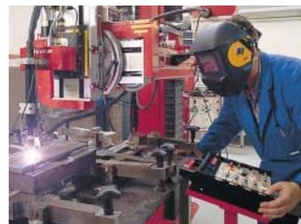
In the welding laboratory at Altena, the base material's suitability for welding is examined, welding materials are developed and tested, and new processes are screened for their transferability to Krupp VDM high-performance materials.
