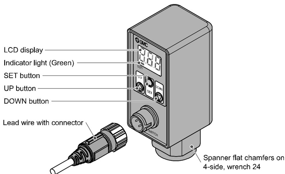
**Indicator light (Green):** Displays the operation condition of the Pressure switch. Lights ON when the output (OUT1) is turned ON.
