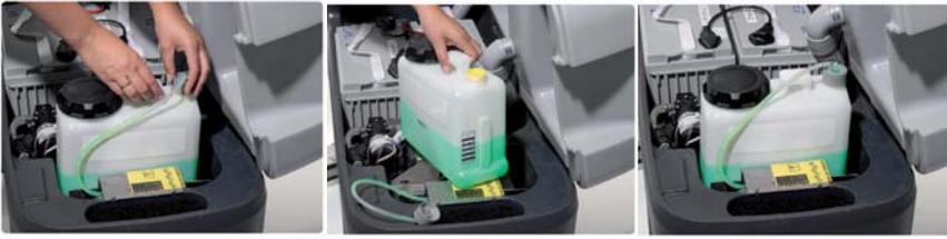
Change of EDS cartridge can be made in a matter of seconds.
