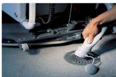
Splash-control hose prevents spillage while emptying tank.
