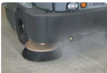
The exclusive DustGuard™ system effectively controls airborne dust by providing a fine mist of moisture to the front and side brushes.
