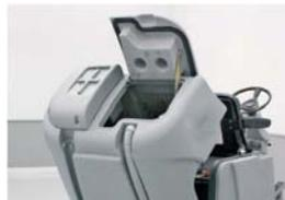
Easy cleaning of tanks and easy access to the batteries
