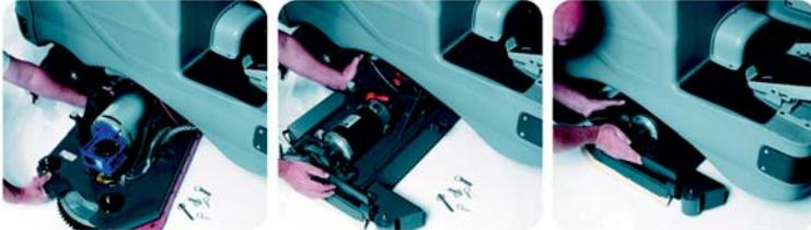
The brush deck can be changed in a matter of seconds by simply removing the holding pins
