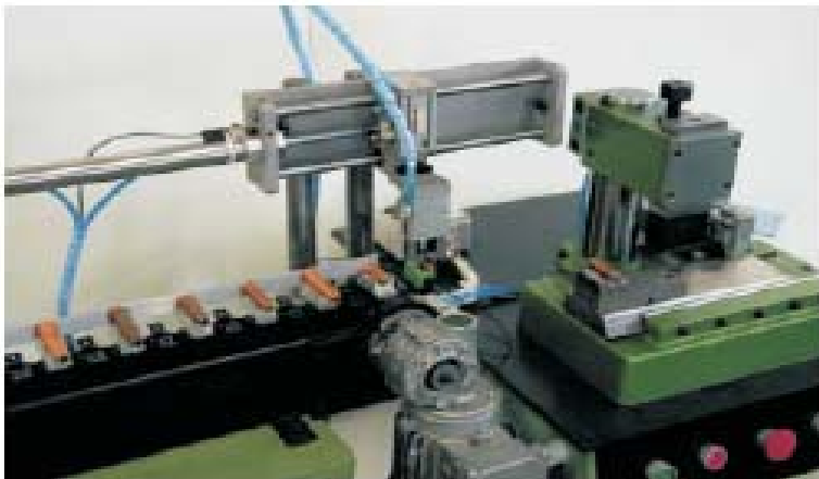
Roller marker MB41E combined with automatic feeding system
