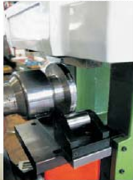
High pressure valve body marked on a MB 76EP
