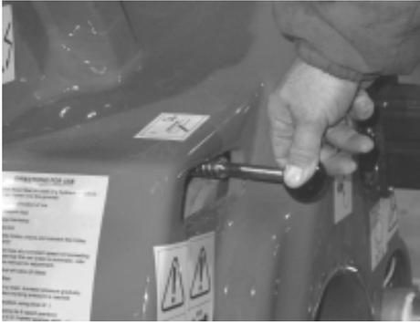
1. Gearbox engage and disengage handle.
