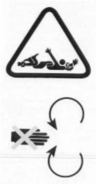
3. This sign indicates dangerous equipment in operation. Never use this machine with safety guards removed. When using a PTO to rewind the hose, use only protected shafts, conforming with the safety standards in force.
