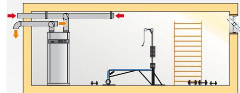
**Variable switching of the intake air:** A pipe duct system with integrated bypass flaps enables variable use of the heat extracted from outdoor or indoor air for hot water preparation.
