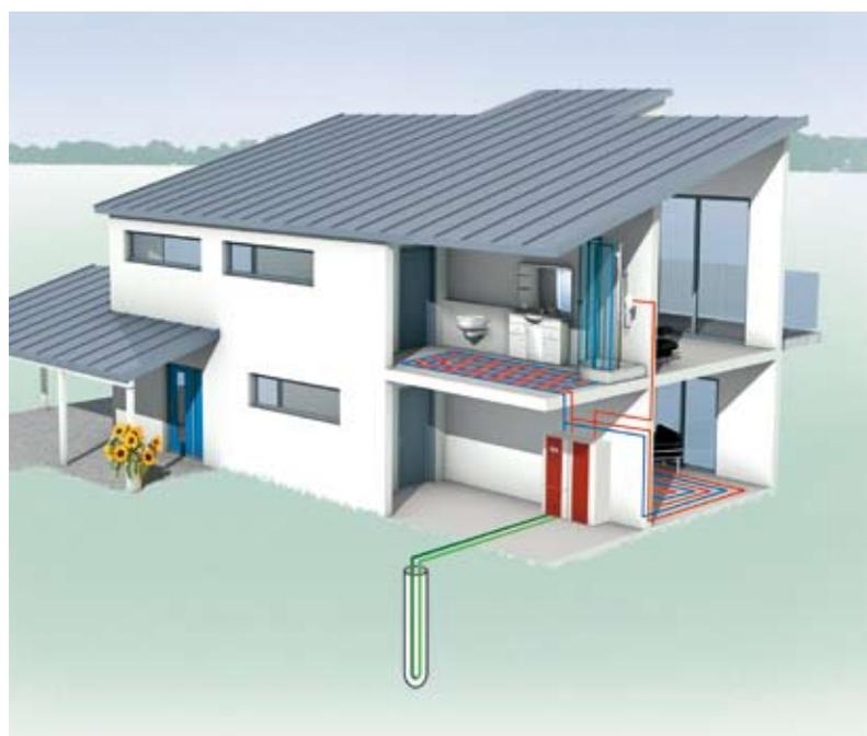
Brine-to-water heat pumps with borehole heat exchangers
