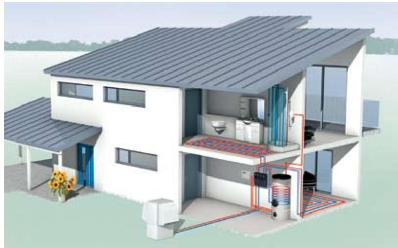
Air-to-water heat pumps for outdoor installation
