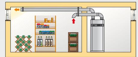
**Cooling in recirculating air operation:** Indoor air is drawn out from storage rooms or wine cellars, for example, via an air duct and is then cooled and dehumidified in the hot water heat pump and blown into the room again. Suitable locations for installation include hobby rooms, furnace rooms and laundry rooms. The air ducting in the heated section of the system should be insulated with water-proof insulation to prevent the formation of condensate.
