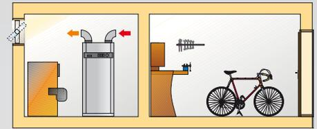
**Waste heat is useful:** Our standard heat exchangers (AWP 30HLW and BWP 30HLW only) for hot water heat pumps enable direct connection of a heat generator, e.g. a solar energy system or a boiler.
