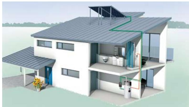
Solar collectors for DHW preparation in combination with the BWP 30HLW and AWP 30HLW hot water heat pumps
