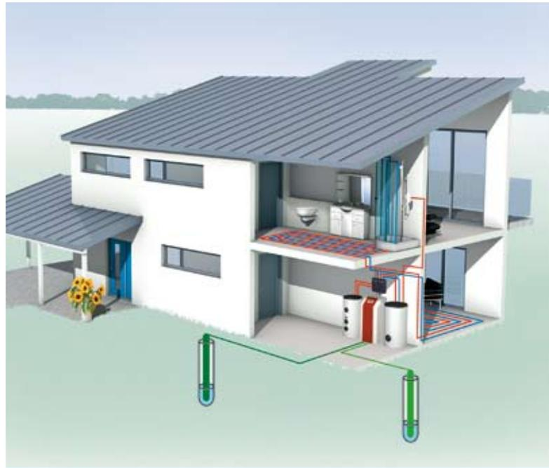
Water-to-water heat pump with well system
