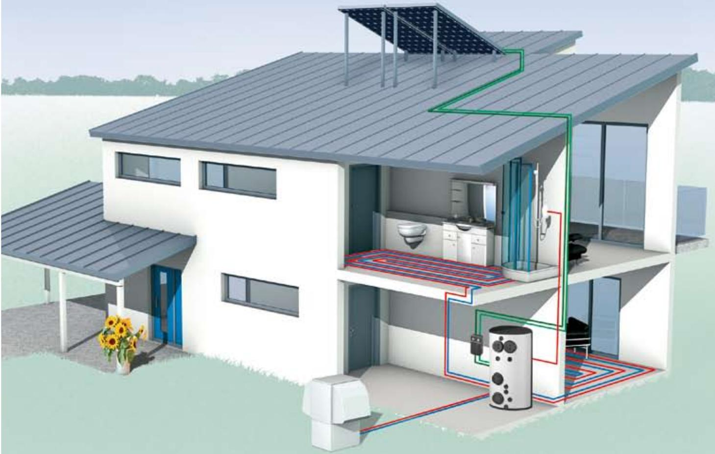
Solar collectors for domestic hot water preparation and supplementary heating in combination with air-to-water heat pumps
