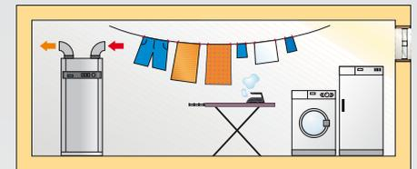
**Dehumidifying in recirculating air operation:** Dehumidified air in laundry rooms can be used to dry laundry and prevents damage caused by dampness.
