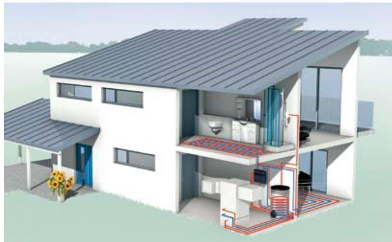
Air-to-water heat pumps for indoor installation
