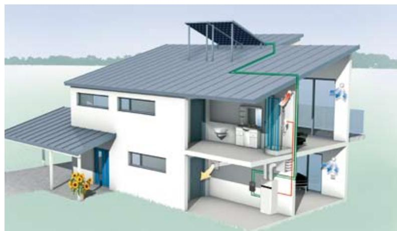
Solar collectors in combination with LWP 300W compact domestic ventilation unit with integrated DHW preparation
