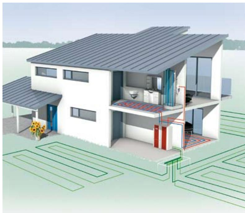
Brine-to-water heat pumps with ground heat collectors
